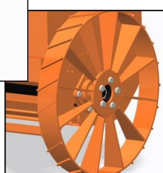
While using with ground wheel on both end of Drum, Wheel can be fitted as show below.
